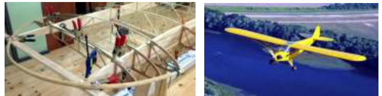
First build-up of the Ailerons and Aileron Brackets and a complete J-3 Piper Cub.
